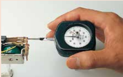
Measurement example of contact force on a relay
