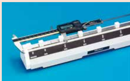
Checking accuracy of caliper (outside measurement)
