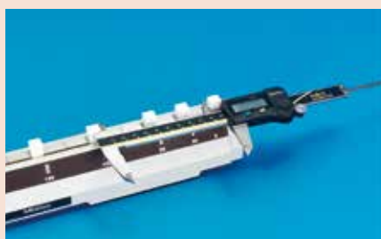
Checking accuracy of caliper (inside measurement)
