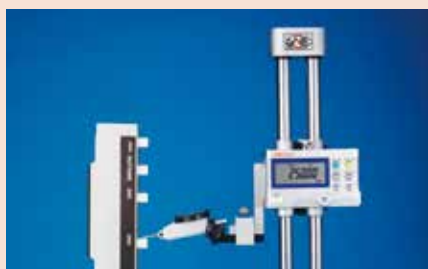
Checking accuracy of height gage
