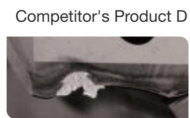
After drilling 18m
