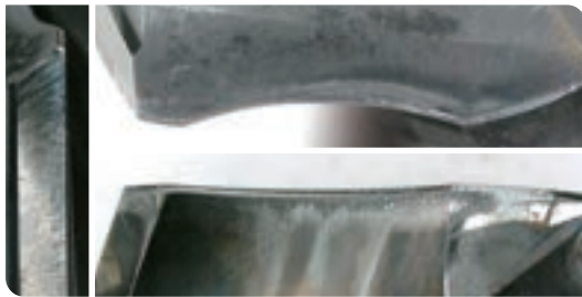
After drilling 2,500 workpieces (5 holes per workpiece)
