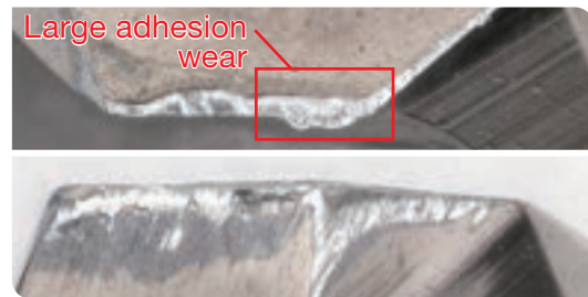
After drilling 900 holes
