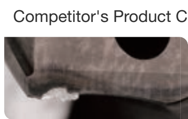
After drilling 21m
