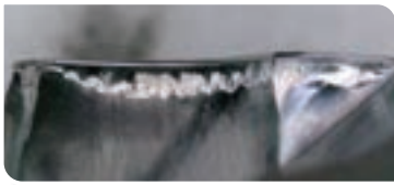
After drilling 46m
