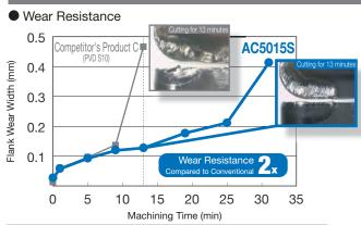
Work Material: Inconel 718 (44HRC) Insert: CNMG120408N-EX Cutting Conditions:  $v_c$ = 40m/min, f= 0.1mm/rev,  $a_p$ = 1.5mm Wet
