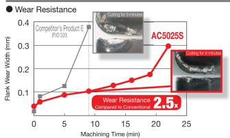
Work Material: Inconel 718 (44HRC) Insert: CNMG120408N-EX Cutting Conditions:  $v_c$ = 40m/min, f= 0.1mm/rev,  $a_p$ = 1.5mm Wet
