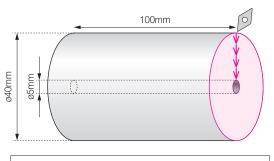
Work Material: SUS304 Insert: DCGT11T302R-FY Cutting Conditions:  $v_c$ = 100m/min, f= 0.05mm/rev,  $a_p$ =0.1mm Wet (oil-based)
