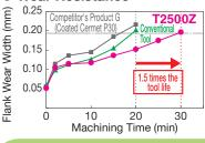
Work Material: SCM435 CNMG120408N-SU Cutting Conditions:  $v_c = 260 \text{m/min}$ f=0.23mm/rev ap= 1.5mm Wet
