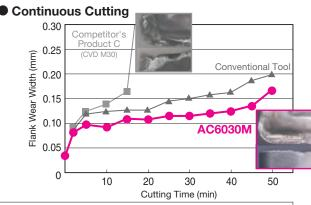
Work Material: SUS316 Insert: CNMG120408N-EX Cutting Conditions:  $v_c$ =200m/min, f=0.2mm/rev,  $a_p$ =2.0mm Wet
