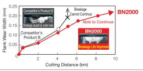
Work Material: SCM415H Round Bar (58 to 62HRC) Insert: 2NU-CNGA120408 Cutting Conditions: v<sub>c</sub>=100m/min, f=0.1mm/rev, a<sub>p</sub>=0.2mm Dry
