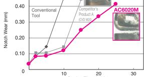
Work Material: SUS316L Insert: CNMG120408N-GU Cutting Conditions:  $v_c$ = 150m/min, f= 0.3mm/rev,  $a_p$ = 2.0mm Wet
