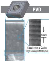
Our proprietary super multi-layered coating structure: Advanced nanotechnology enables nanometre-level thickness (1 nanometre is one billionth of a metre). Hardness, thermal resistance and toughness are significantly improved by alternately layering one thousand layers of super thin film
