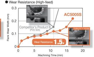
Work Material: Inconel 718 (44HRC) Insert: CNMG120408N-EG Cutting Conditions:  $v_c$ = 50m/min, f= 0.25mm/rev,  $a_p$ = 1.2mm, Wet
