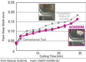
Cutting Conditions:  $v_c$ = 200m/min, f= 0.3mm/rev,  $a_p$ = 2.0mm Wet
