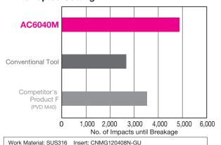
Cutting Conditions: vc=230m/min, f=0.23mm/rev, ap=0.8mm Dry
