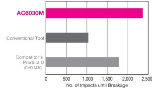
Work Material: SUS316 Insert: CNMG120408N-GU Cutting Conditions:  $v_c$ =100m/min, f=0.1mm/rev,  $a_p$ =1.0mm Wet
