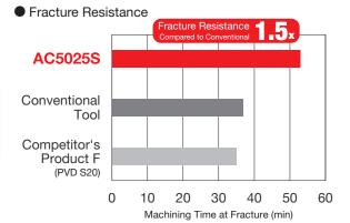
Work Material: Hastelloy (22HRC) Insert: CNMG120408N-EX Cutting Conditions:  $v_c$ = 50m/min, f= 0.1mm/rev,  $a_p$ = 1.5mm Wet
